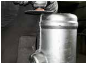
Grinding of cast parts
